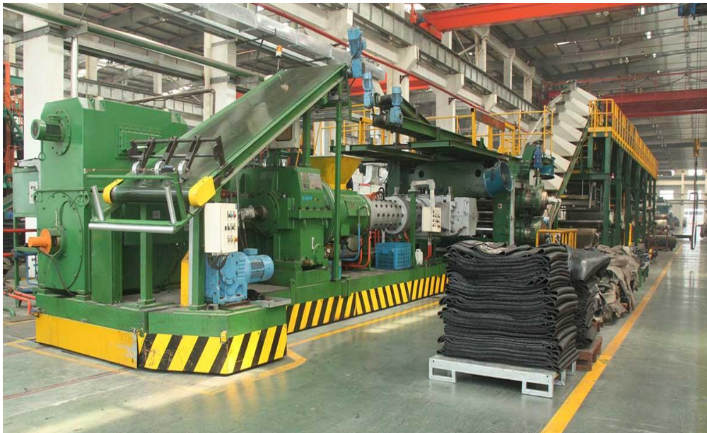
b) Production line of wide extruded calendaring rubber sheet 1
